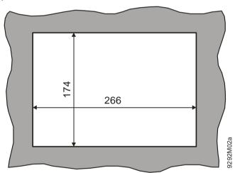
Wall thickness: 1 mm to 4 mm
