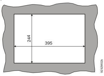
Wall thickness: 1 mm to 4 mm
